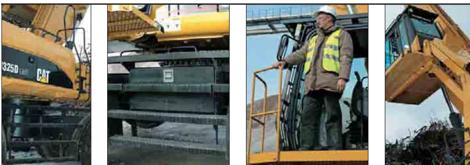
Cab Access System. The M325D MH and M325D LMH can be equipped with a newly designed cab access system. This cab features an additional cab platform with handrails located to provide the operator with safe ingress and egress.
